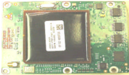
GB-GRAM measures 3.4 X 2.4 inches and weighs in at 3.5 ounces.
