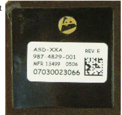
Okay, its not much to look at but even at less than 2 square inches, the current SAASM is the “heart” of a military GPS receiver!
